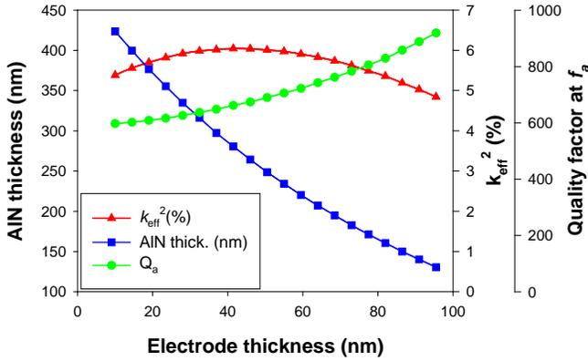
Figure 3. AIN thickness (■),  $k_{\text{eff}}^2$  (▲), and  $Q_a$  (●) vs Ir bottom electrode thickness. Simulations were made for resonators tuned at 8 GHz and AIN layers with  $k_{\text{mat}}^2$  of 6.5%. Acoustic losses in AIN were considered.
