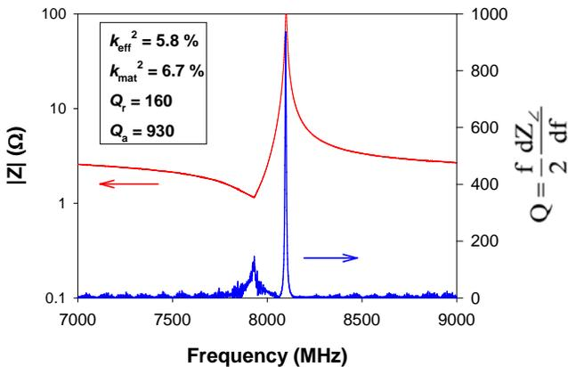
Figure 4. Impedance modulus and  $Q$  as a function of frequency.
