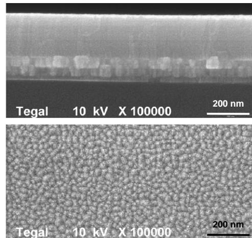
Figure 2. Cross-section and plane-view SEM images of a typical 200 nm-thick AlN film.
