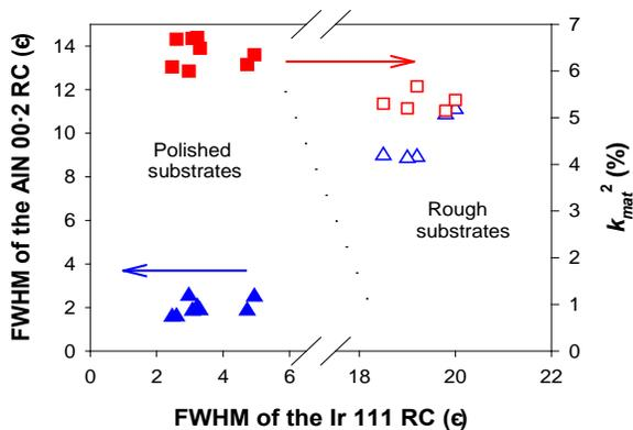
Figure 1. RC around the (00-2) AlN XRD peak (▲) and  $k_{mat}^2$  (■) as a function of the RC around the (111) Ir peak.
