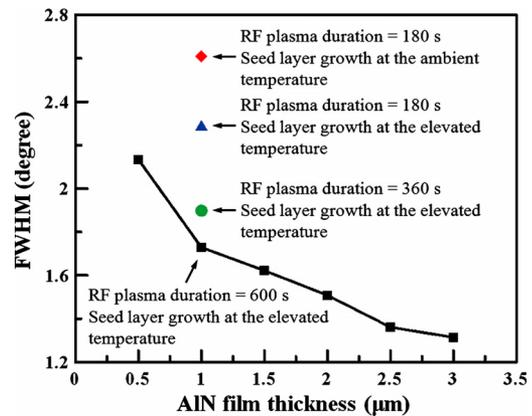
FIG. 2. (Color online) Plot of the measured FWHM of AlN thin films grown under different deposition conditions vs AlN film thicknesses.
