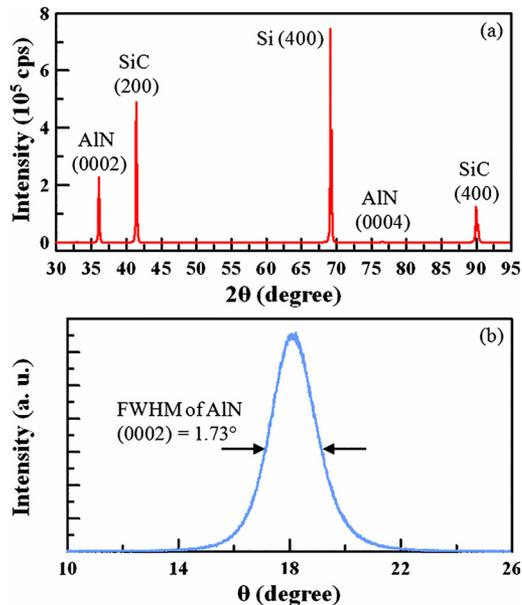
FIG. 1. (Color online) (a) XRD spectrum of the AlN(0002)/3C-SiC(100)/Si(100) layered structure where the AlN film is 1  $\mu\text{m}$  and the 3C-SiC layer is 2.3  $\mu\text{m}$ . (b) Rocking curve of 1- $\mu\text{m}$ -thick AlN (0002) film deposited on the epitaxial 3C-SiC layer on the Si (100) substrate.
