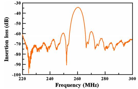
FIG. 4. (Color online) Measured frequency responses of the SAW device on the AlN/3C-SiC/Si layered structure after time-gating.
